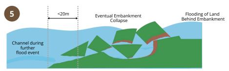
The overhanging bank material continues to be eroded during repeated flood events, which are becoming increasingly common due to climate change, and the ever growing burden of overhanging material eventually leads to the collapse of the embankment.
