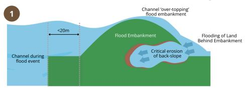
Flood embankments <20m from the water's edge are most at risk of collapse due to water rising over the bank and quickly eroding its backslope, known as 'over-topping'. Of 228 breaches between 1990 to 1998 in the Tay catchment, 97% were due to 'over-topping'.
