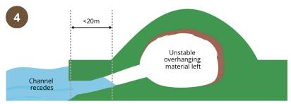
When the water level recedes the vacated beaver burrow is enlarged, 'weakening' the embankment leaving overhanging bank material.
