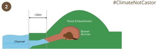
Weakening' originating from wildlife burrows, such as those created by beavers, are a minor cause of embankment collapse. A beaver burrow on its own is also unlikely to be large enough to destabilise an embankment causing it to collapse.
