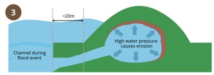
During flood events, beavers vacate as water levels rise. The high water pressure within the flooded burrow causes erosion.
