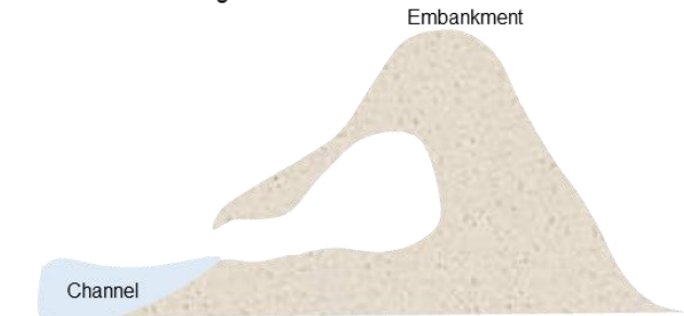
4. The beaver burrow is enlarged, weakening the embankment leaving overhanging bank material.
